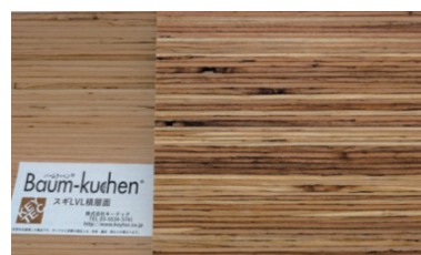
Example of coating with bio-based paint designed for soft feel and improved durability (used on construction plywood)
